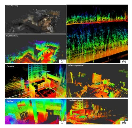
Fig. 3 Point clouds captured by WHU-Helmet. (a) Ancient building; (b) Urban vegetation; (c) Outdoor and indoor 3D mapping. (d) Aboveground and underground 3D mapping.
