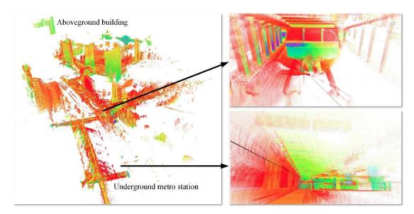
Fig. 2 3D mapping of the urban underground space.
