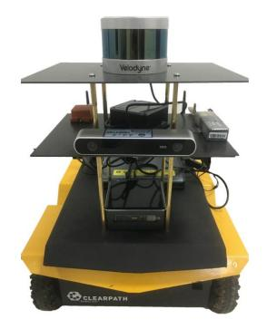
Fig. 4 UGV 3D mapping system.
