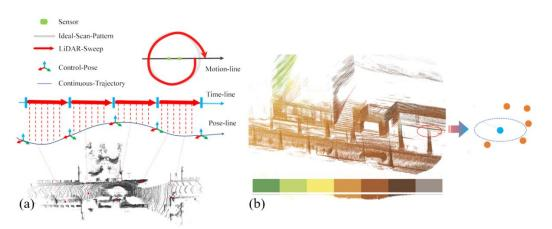
Fig. 5 3D-CSTM system. (a) spline based non-rigid registration; (b) continuous time and spatial mapping (color encodes time-stamp).
