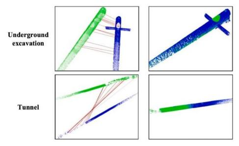
Fig. 6 JoKDNet for registration of underground point clouds.
